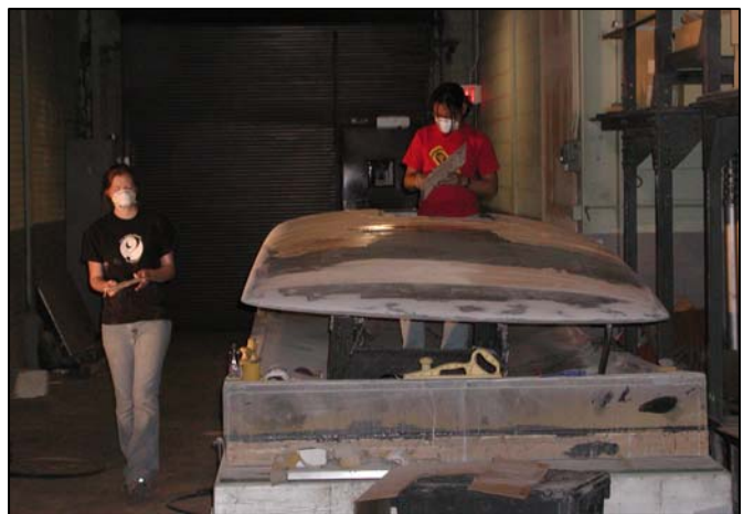
Mech Team members Sarah and Hilda working on Fusion's show shell. Although the part looked acceptable coming out of the molds, we want to smooth out even the smallest defects on the show shell.
