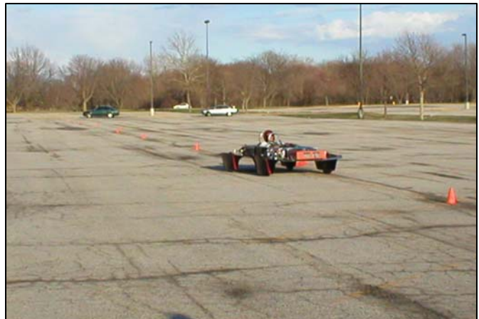
Fusion running the slalom in the Hilton Coliseum for the first time. Drivers reported significant improvement over Spectrum's handling performance during higher speed maneuvering.
