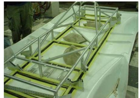
Assembling of manufactured parts to get a finished product
